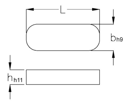
$\begin{array}{ll} b & = 8 \\ h & = 7 \\ L & = 70.0 \\ Tolerance \ b = 0.036 \\ Tolerance \ h = 0.090 \\ Tolerance \ L = -0,3 \end{array}$
